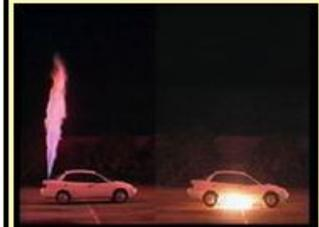
Photo 2 - Time 0 min, 3 seconds - Ignition of both fuels occur. Hydrogen flow rate 2100 SCFM. Gasoline flow rate 650 cc/min.
